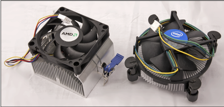
Figure 1-4 Manufacturer-supplied heat sinks for AMD (left) and Intel (right) CPUs.
